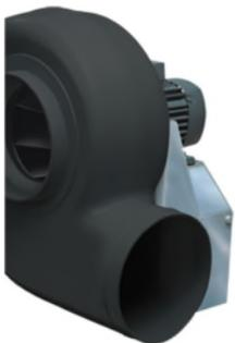
The casings are produced following the rotational casting procedure and are made of electrically conductible nonflammable grey polypropylene (PPs-el). The design allows to remove the motor-impeller-unit and the console without disconnecting casing from the duct system. Casing and special steel console are sealed with an expanded PE-sealing.
