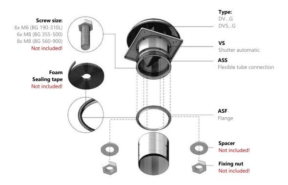
**Step 4**Installation Flat roof socket
