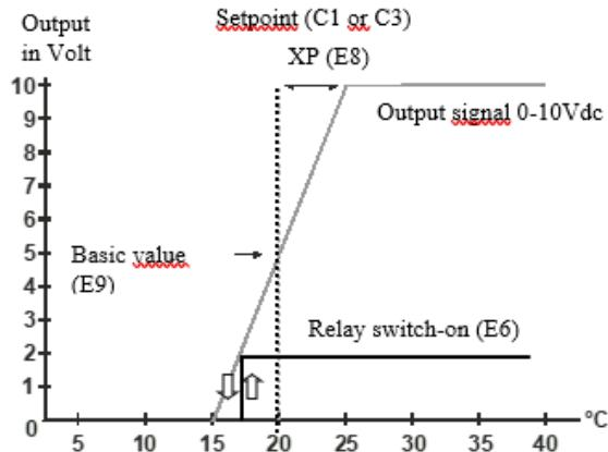
Picture: Representation of control loop with inverted effective operating direction at reference variable temperature. The measured reference variable temperature shown in the figure increases, and the control output (the actuated variable) rises.
